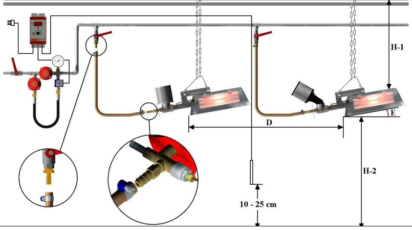
Installation height H-1: we recommend an open space above the M8 of 100cm or more. (60cm is the minimum and this is for a non-burnable ceiling only!) installation height H-2: we recommend installing the heaters 90-150cm from the ground. If the heaters are higher, they will cover a larger area. For colder conditions we would install the heaters lower. Angle E= check installation manual. D is spacing < 7m, depending on the conditions.
